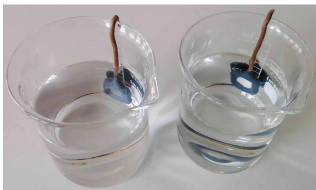
Fig. 1. Specimens immersed in artificial saliva
