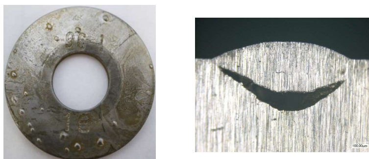
Figure 21. Coupon after 330 days of exposure to vapors from second-stage hydrodesulfurization (HDS) reaction.
