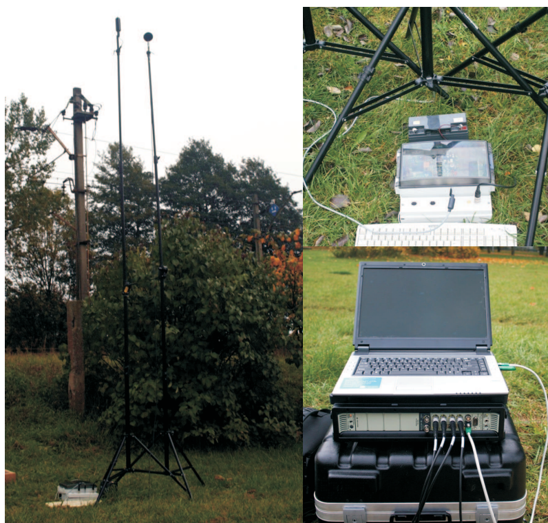
Fig. 9. Engineered monitoring station and PULSE system employed to short-term outdoor measurements.
