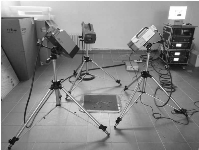
Figure 8. Polytec PSV-400-3D laser scanning vibrometry unit used for experimental tests.
