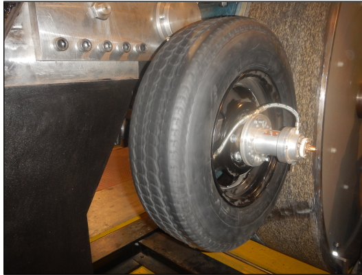
Figure 3: Roadwheel facility with 2.0 m diameter drum at the Technical University of Gdańsk, Poland
