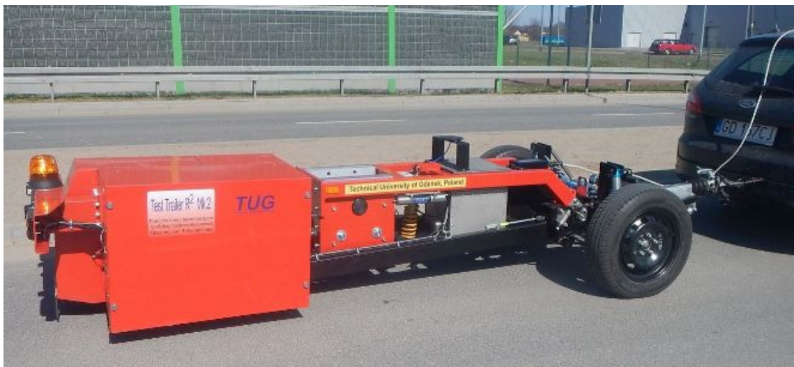
Figure 2. Rolling Resistance test trailer R^2 Mk.2.
