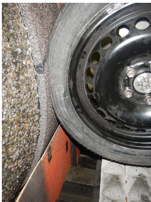
Figure 1. Roadwheel facility at the Technical University of Gdańsk equipped with replica road surfaces.
