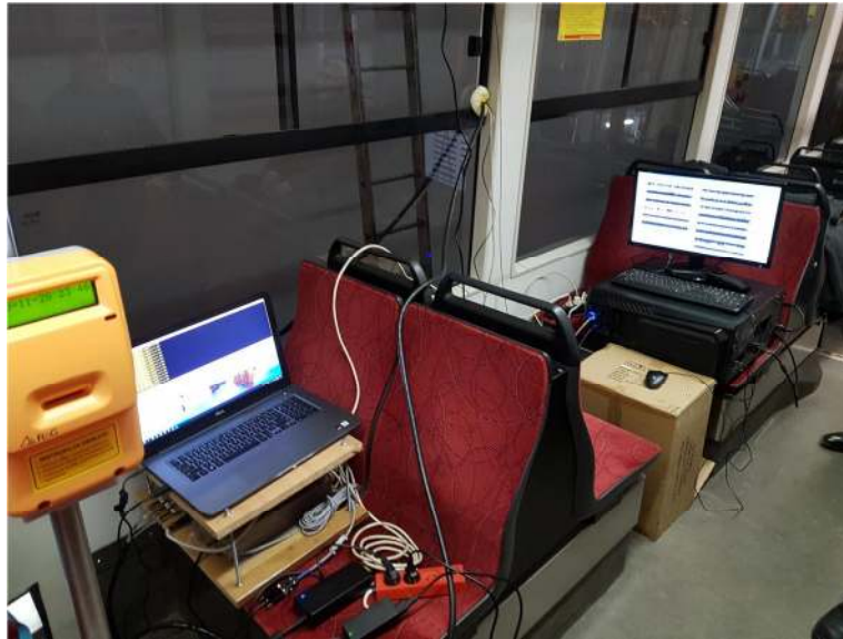
10. Accelerometer and inclinometer system and GNSS compass controllers
