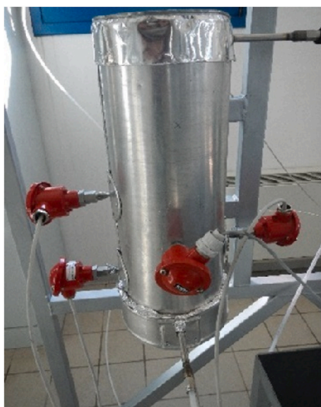
Fig. 3. Customized shaft furnace.
