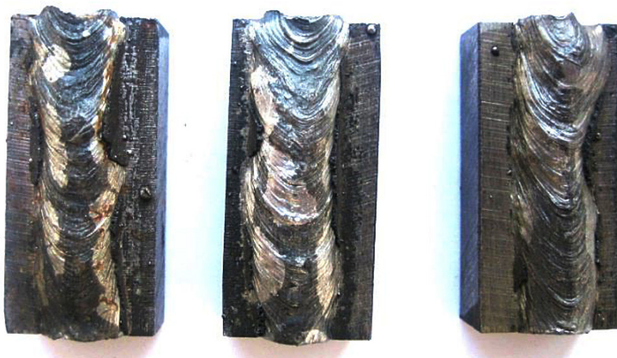
Figure 9. Specimens for determination of diffusible hydrogen content in deposited metal
