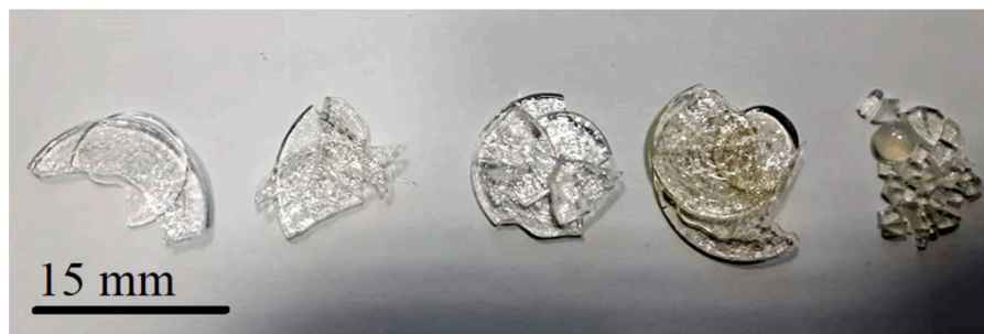
Fig. 2. Photograph of the as-quenched samples: 0Nb, 0.8Nb, 1.4Nb, 1.8Nb, and 3.4Nb (from left to right).
