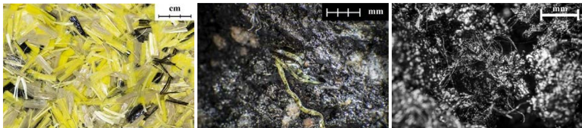
Fig. 1. a) Loose fibres, b) Fibres in laboratory mixed asphalt concrete, c) Fibres in plant mixed asphalt concrete, (all photos by Ł.Mejlun).
