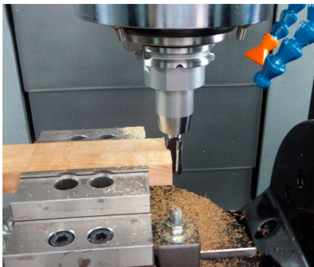
Figure 4. Machine tool AX320 Pinnacle with equipment for machining tests.
