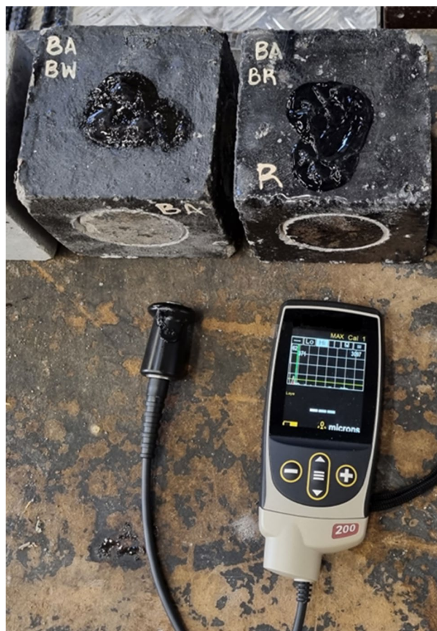
Figure 3. Measurement of coating material thickness.
