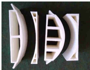
Fig. 4. The forms used for bending the investigated EDLC specimens
