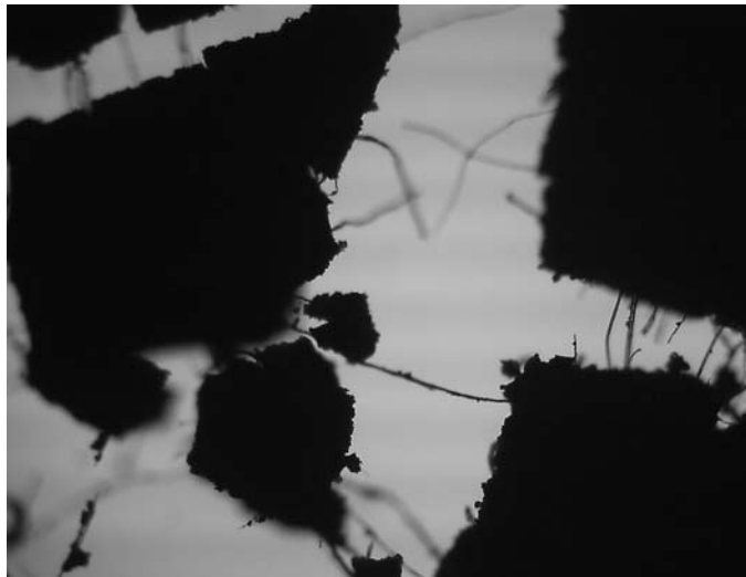
Fig. 4. Sediment from backwashing filters – in the form of dried broken cake. Magnification 40x
