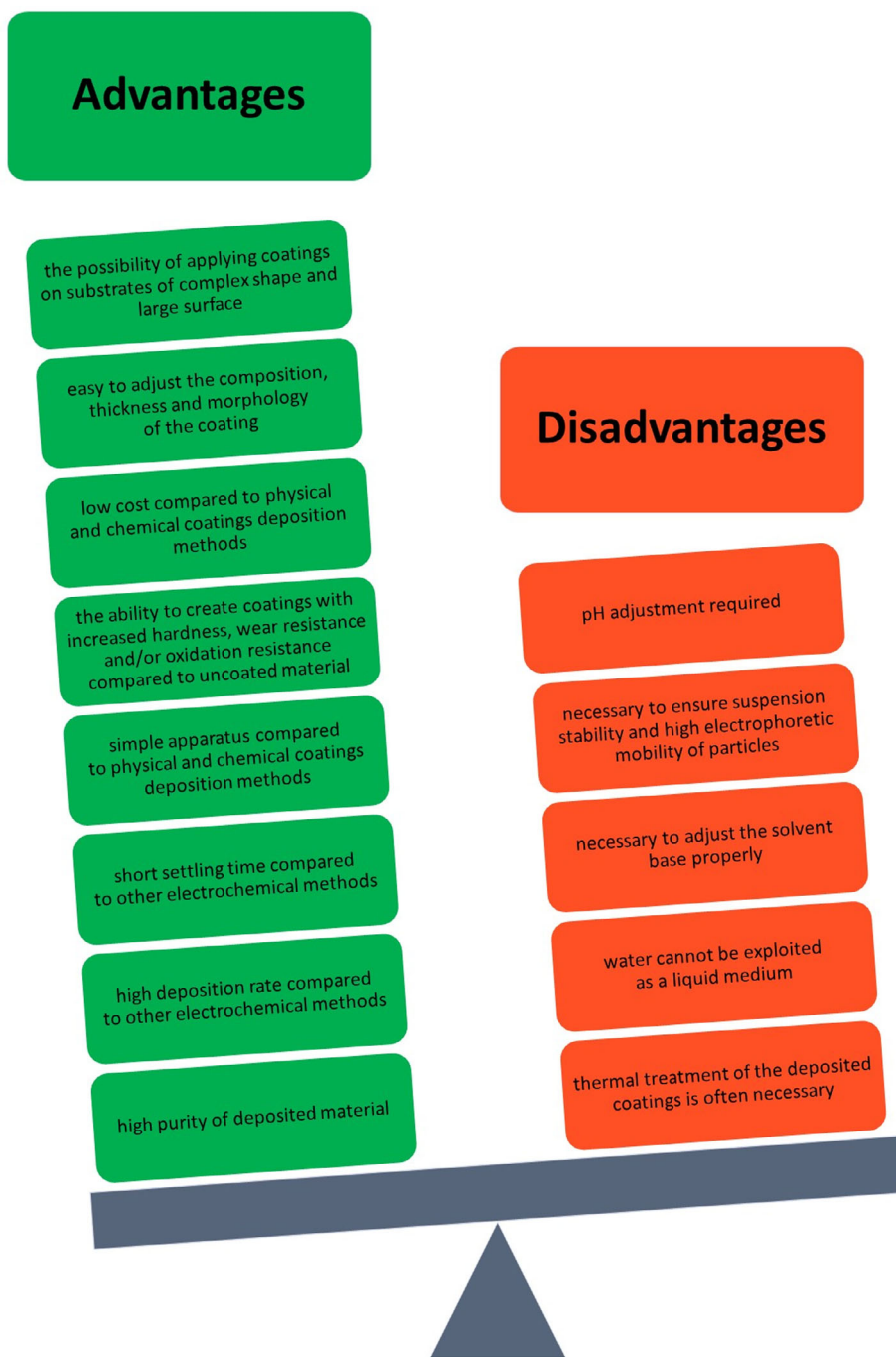
FIGURE 1 Advantages and disadvantages of the electrophoretic deposition method in respect of biomedical applications. 38-41,47 Designed and illustrated by the authors of this work.
