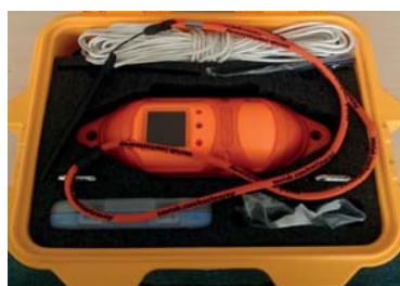
Fig. 11. Sonic sounder for measuring sound speed
