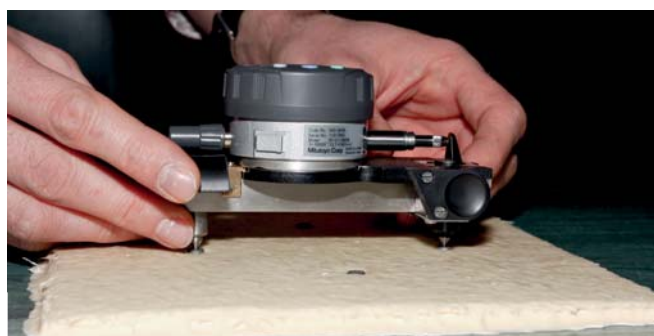
Fig. 5. Extensometer used for length change measurement
