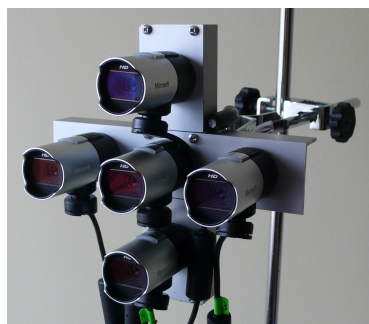
Figure 3. The camera set consisting of MS LifeCam Studio mounted in the form of Equal Baseline Camera Array.
