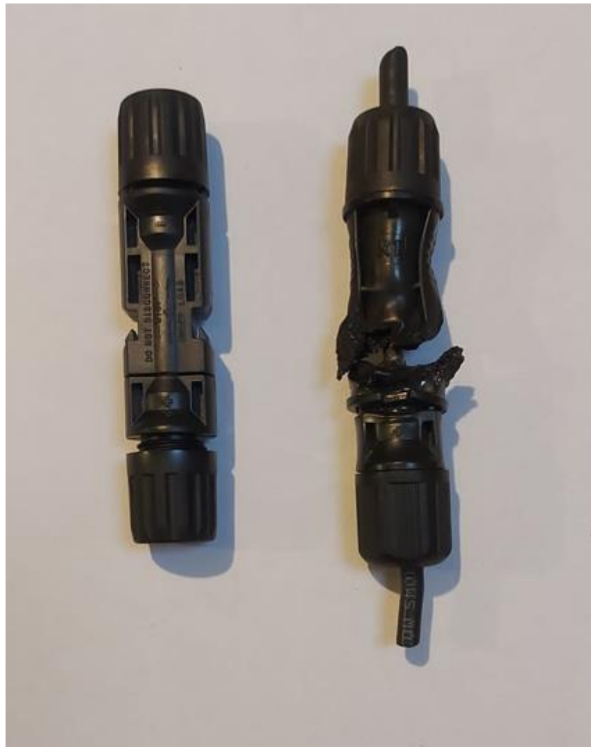
Figure 13. Comparison of the shape of MC4 connectors—the connector on the left is fully functional and the connector on the right is damaged due to overheating.
