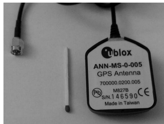
Figure 2. u-blox GPS Antenna with magnetic base.
