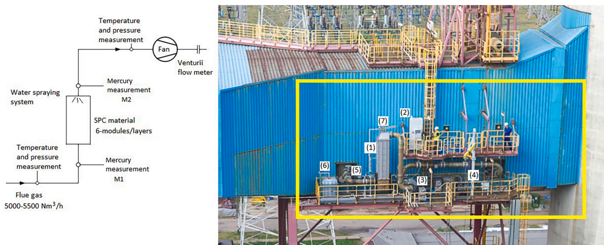
Fig. 4. Industrial scale test rig: scheme (left) and photo (right). In the photo: 1 – SPC modules, 2 – mercury measurement (GASMET), 3 – fan, 4 – Venturi, 5 – flue gas bypass, 6 – water tank, 7 – water spraying system.
