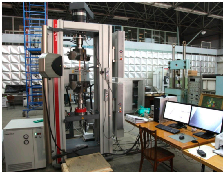
Figure 2. A General view of the testing setup Z100 ZWICK-ROEL.
