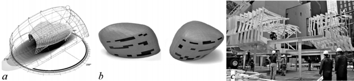
Fig. 3. (a) solar analysis, (b) envelope optimization, (c) structure assembly.
