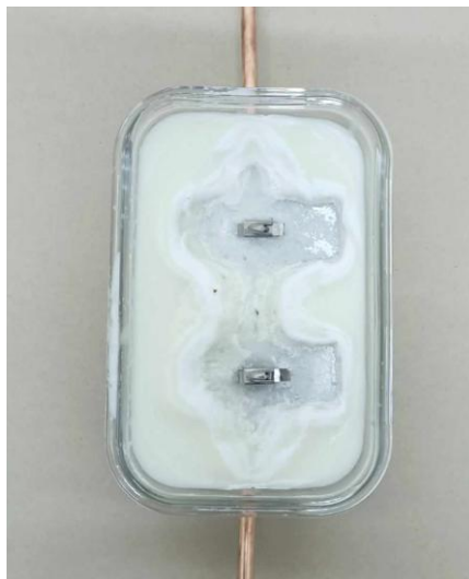
Fig. 9. Visible left-out liquid and solid phase boundaries after solidification of the soy wax.
