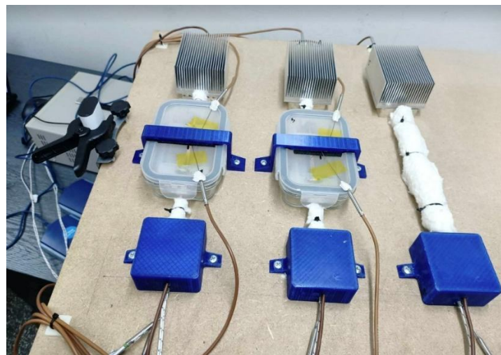
Fig. 3. The experimental stand for investigating PCM-assisted HPs for electronics cooling. Two rigs are for testing lauric acid and soy wax, the third being a reference.
