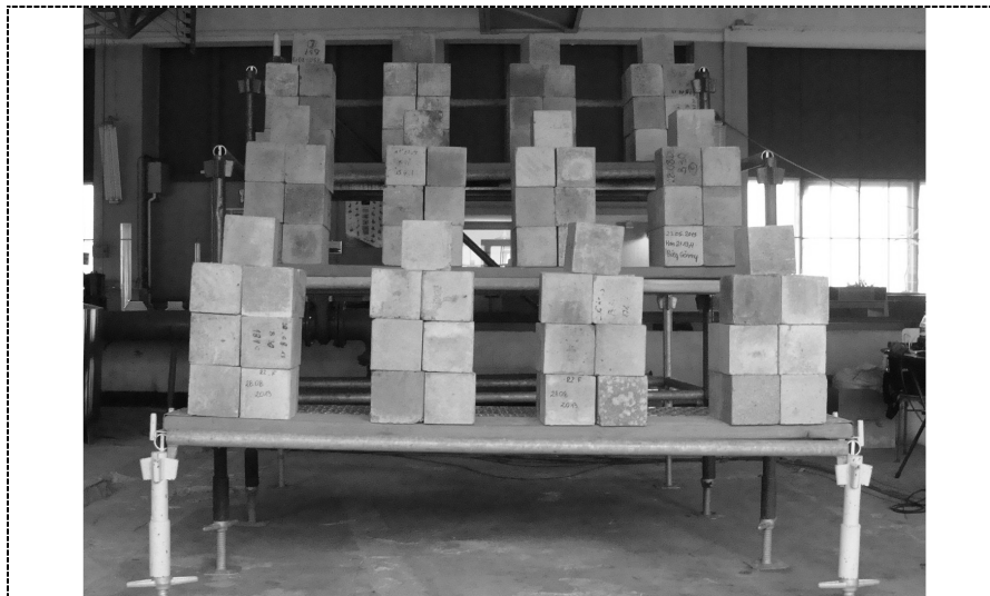
Figure 4. Front view of occupied steel temporary grandstand.
