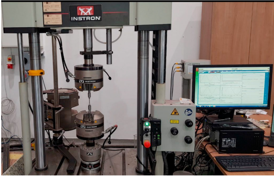
Fig. 3. Universal testing system Instron 8802.
