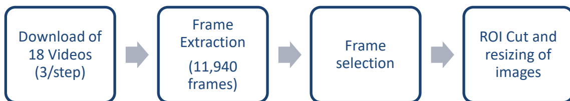
Figure 2: Video processing flow.
