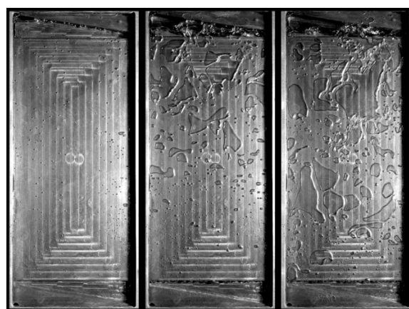
Figure 21. Flow boiling structures of ethanol for a different average wall superheating degree: Left = 1.53 K; middle = 13.22 K; right = 16.2 K.
