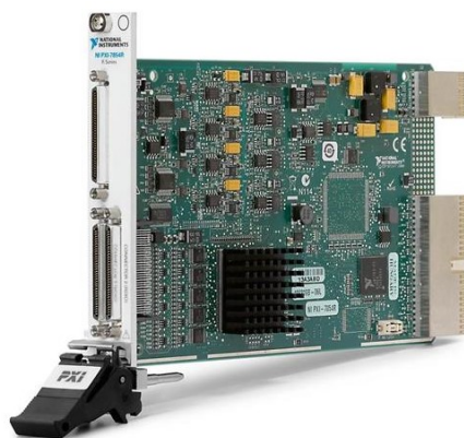
Figure 1. Field-Programmable Gate Array (FPGA) PXI-7854R illustration [11].
