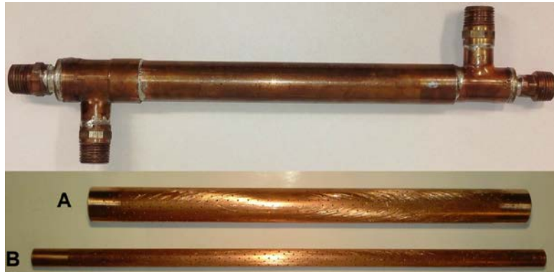
Figure 2 View of MJHE and its perforating pipe of hot fluid (A) and cold fluid (B).
