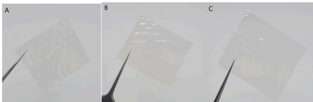
Fig. 1. Digital images of the obtained films A) 80HA/20TA, B) 50HA/50TA, C) 20HA/80TA.
