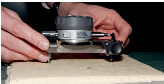
Fig. 5. Extensometer used for length change measurement
