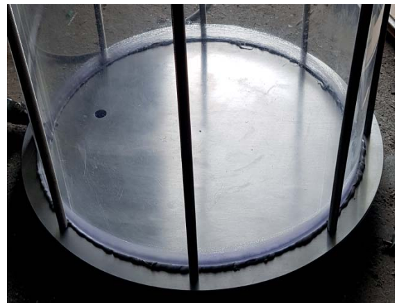
Fig. 8. Sealing of lower tank
