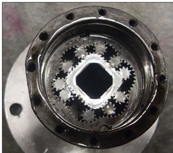
Figure 16. The destroyed satellite mechanism.
