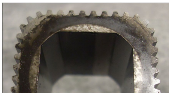
Figure 29. A layer of burnt rapeseed oil on the rotor surface (left) and the characteristic purple layer on the commutation plate (right) —after 3237 min of operation.
