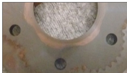
Figure 29. A layer of burnt rapeseed oil on the rotor surface (left) and the characteristic purple layer on the commutation plate (right) —after 3237 min of operation.
