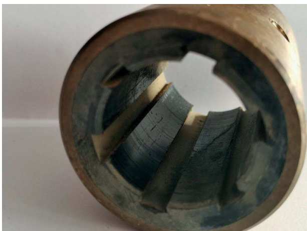
Fig. 5. The PTFE sliding bush (B)
