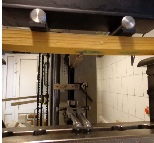
Figure 3. The 4-point bending tests - location of the sensor arms
