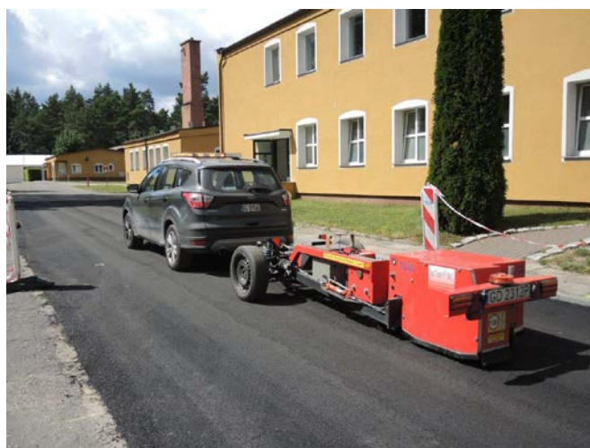
Figure 25. Test trailer R 2 Mk.2 during measurements of rolling resistance on the Dąbrówka test section.
