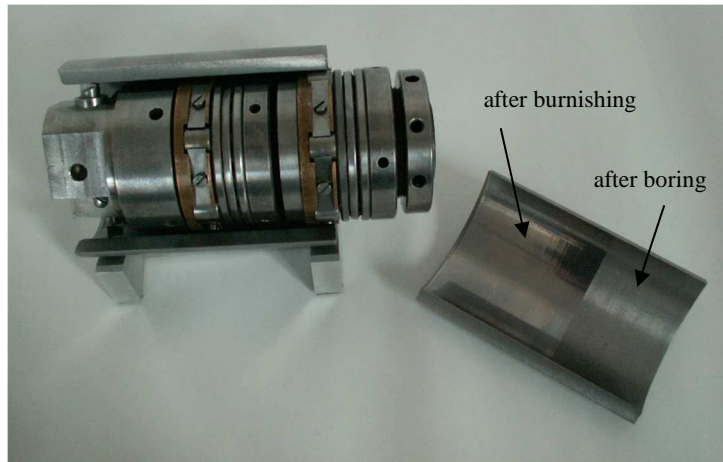
Fig. 7. A view of the boring-burnishing head in the hydraulic cylinder and a cylinder segment before and after machining
