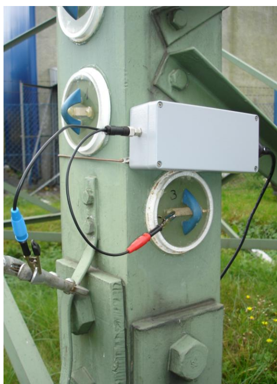
Fig. 1. a) The photography of cells for impedance measurement of anticorrosion coatings on a high-voltage pylon b) Cross-section of the anticorrosion coating and the measurement cell
