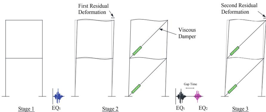
**Fig. 2.** Proposed computational method for retrofitting damaged buildings.
