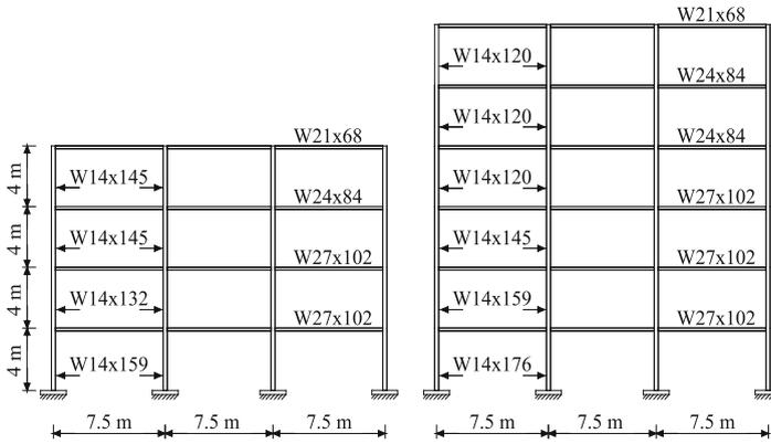
**Fig. 1.** Structural details of the 4-, and 6-Story frames.
