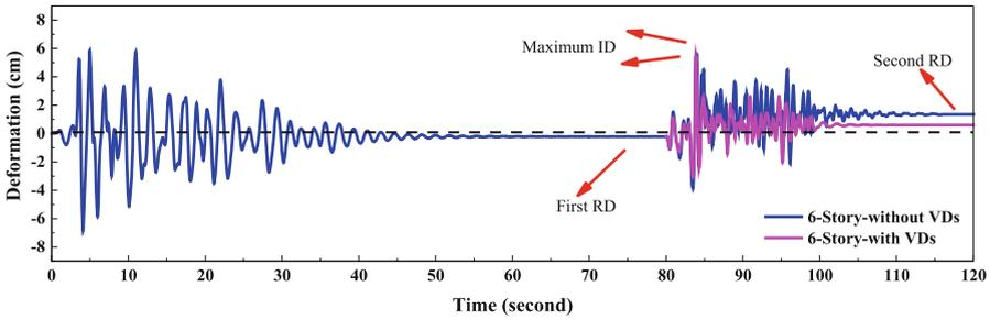
**Fig. 4.** Comparing the deformation results of the 6-Story frame in the seismic mainshock-aftershock analysis with and without VDs.
