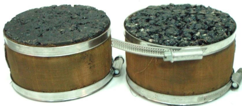
Figure 3. Image of specimens prepared for long-term aging testing.
