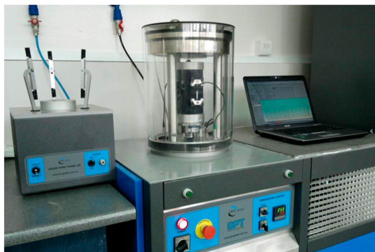
Figure 1. Image of the Asphalt Mixture Performance Tester/Simple Performance Test (AMPT/SPT) equipment IPC Global, Boronia, Australia.
