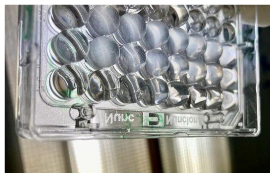
Fig. 4 - Prepared well plate with a McFarland calibrated bacterial suspension prior to rocket launch.
