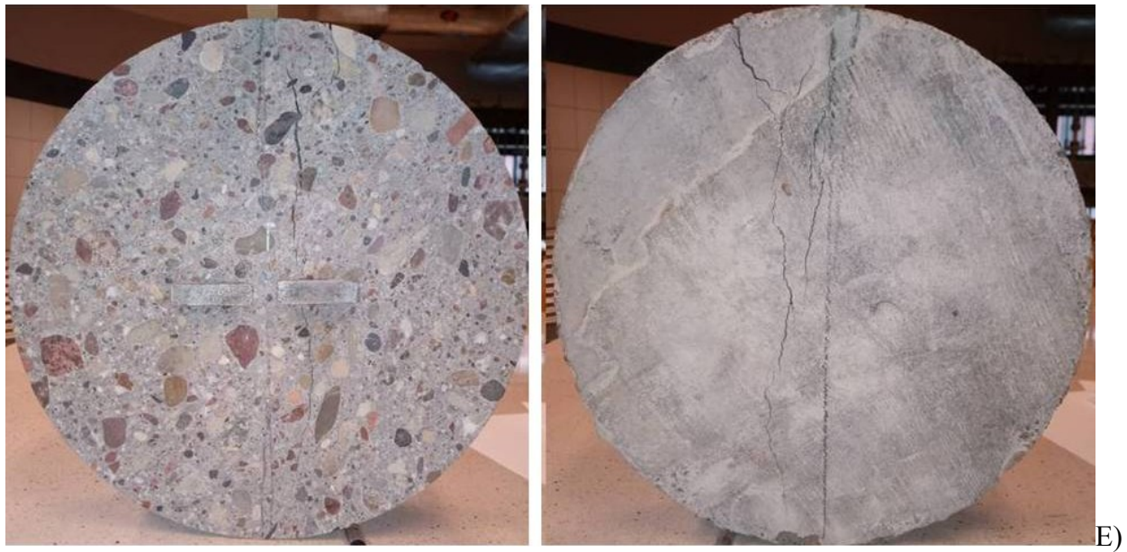
Fig.3.29: The crack patterns for specimens diameters A) D=74 mm, B) D=100 mm, C) D=150 mm, D) D=192 mm and E) D=250 mm for each tested specimen
