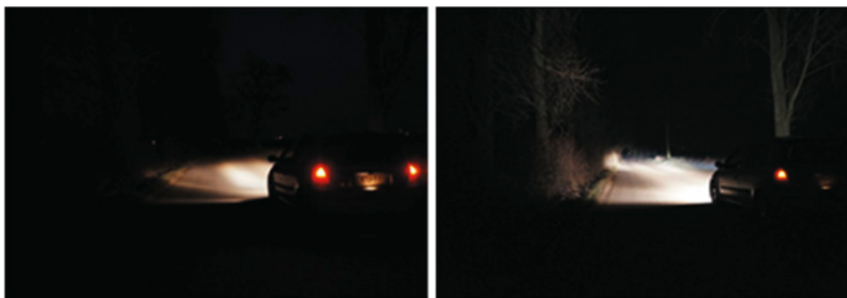
Fig. 4. Comparison between the road illumination by dipped-beam and main-beam headlamps (by: Krzysztof Stryjek)
