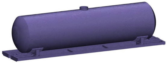
Fig. 9. A finite-element model of the bearing structure of a tank car
