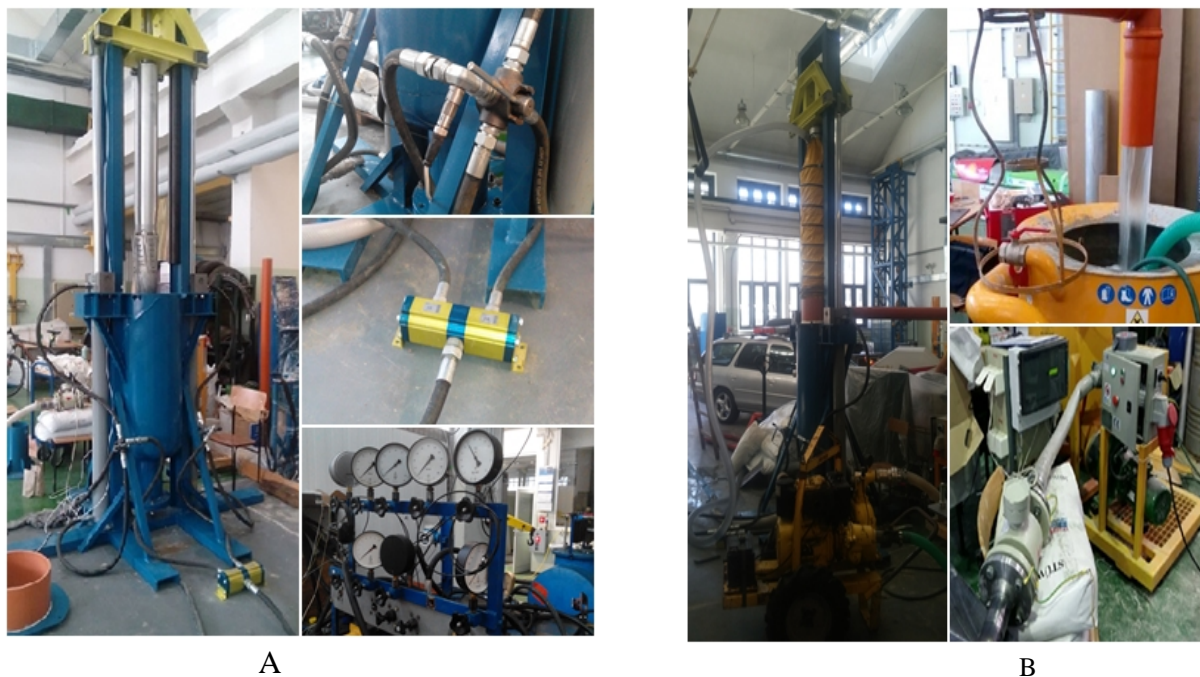
Fig. 7. Clay-cutting laboratory testing station at Gdansk University of Tehcnology: A – hydraulic system, B – mud circulation system.
