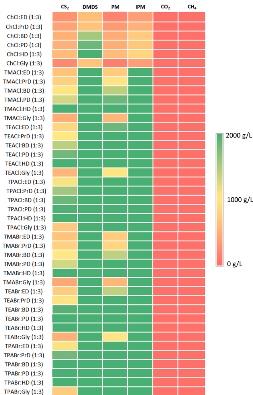
Fig. 2. Matrix of solubility screening of volatile organosulfur compounds, CH 4 , and CO 2 in DES based on COSMO-RS model.
