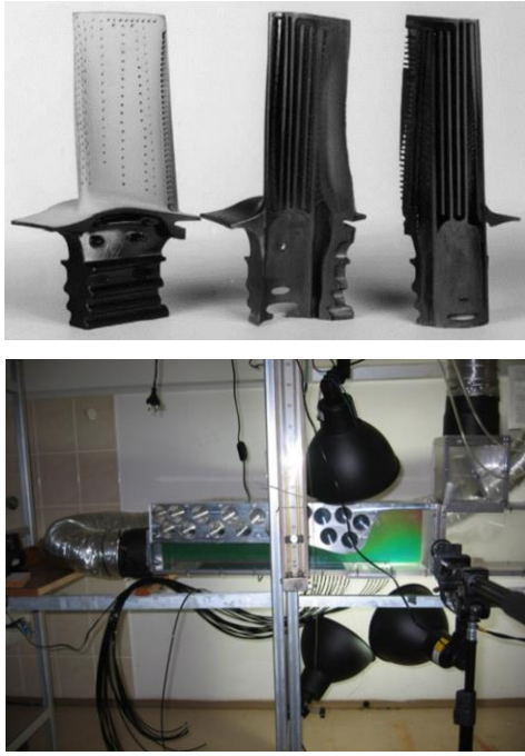
Fig. 23. Gas turbine blades with cooling holes (up) and view of the test section for the model turbine blade cooling system (down) [35].
