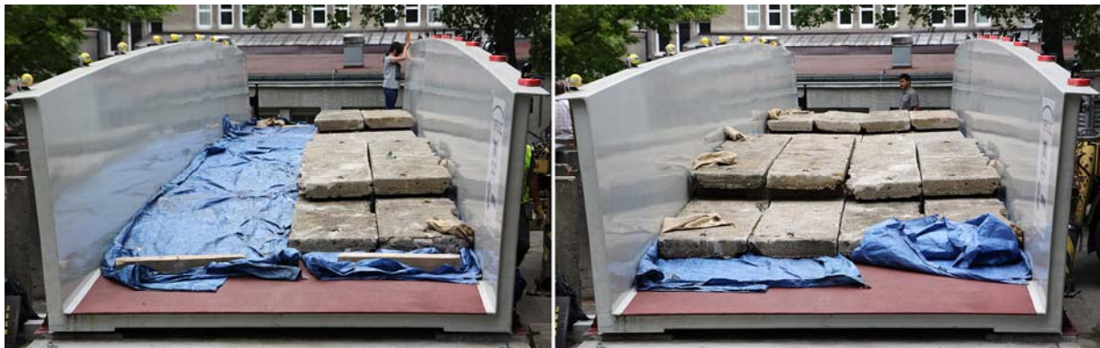
Figure 5. Footbridge loaded with ballast during static tests
