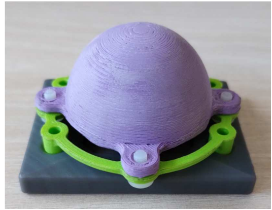
Fig. 3. The antenna array with the 3-D printed PLA lens.
